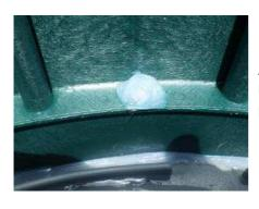
Apply silicone to the screw head to prevent water penetration.
