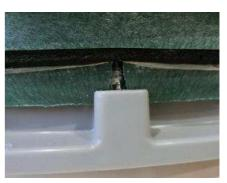
Polylok Risers. Align molded "frame block" with riser screw hole. Insert screw and screw tight. Maximum screw length is  $1 \frac{1}{4}$ "
