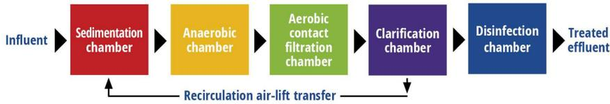
**Two Air Lift Pumps.** One Recirculating Air Lift pump sending process water and solids back to Chamber 1, and one Effluent Air Lift Pump for measured discharge of treated effluent. (See airlift pump info below).
