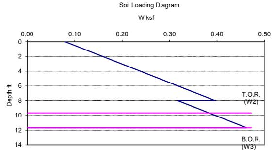
Horizontal lines indicate top & bottom of riser wall
